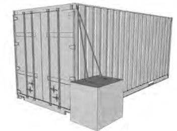
External Ballast Pre-Cast Concrete Block
