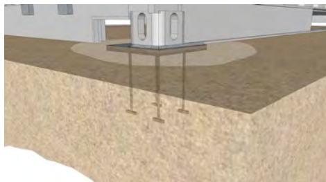
Concrete Footing Welded Container Base Plate
