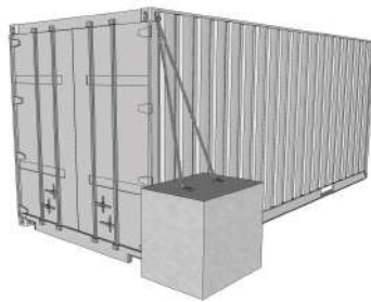
External ballast - pre-cast concrete block
