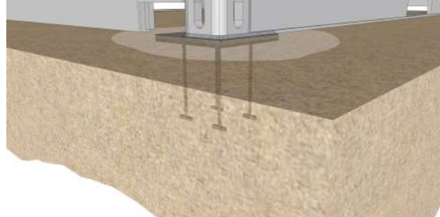
Concrete footing - welded container base plate
