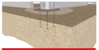
Concrete footing - welded container base plate
