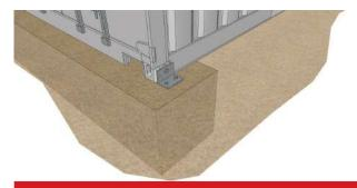
Concrete footing - container hold down bracket
