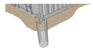
Concrete footing with cast-in chain
